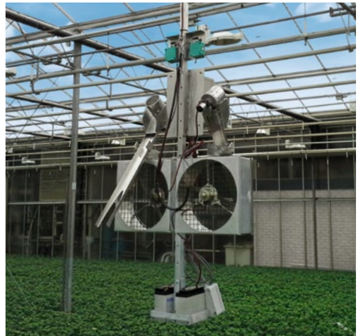
Ultrasonic sensors mounted on either side of the arm ensure reliable collision protection in the greenhouse.
