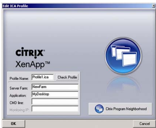
Fig. 2: An ICA profile can be set up with a few mouse clicks: Citrix Program Neighborhood supplies the parameters
